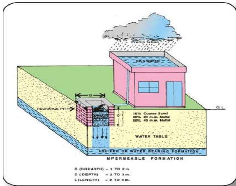
**(b) ROOF TOP RAIN WATER HARVESTING THROUGH RECHARGE TRENCH**
