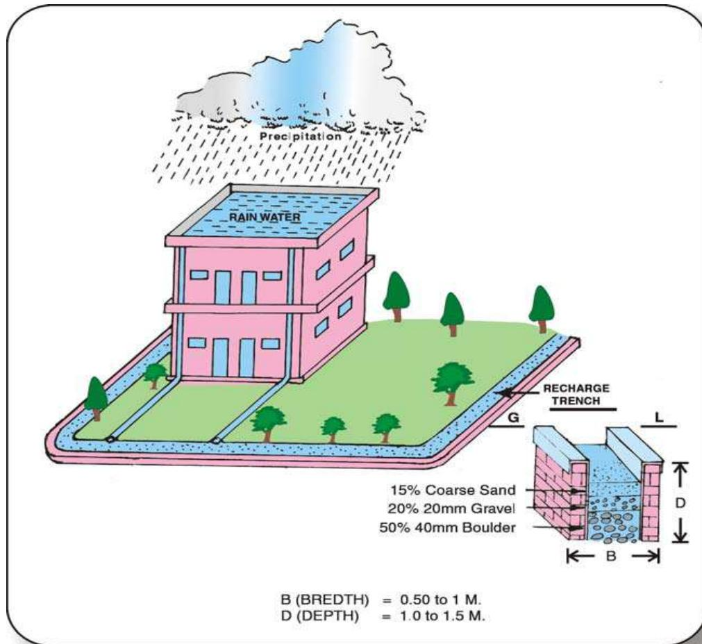
**(c) ROOF TOP RAIN WATER HARVESTING THROUGH EXISTING TUBEWELLS**
