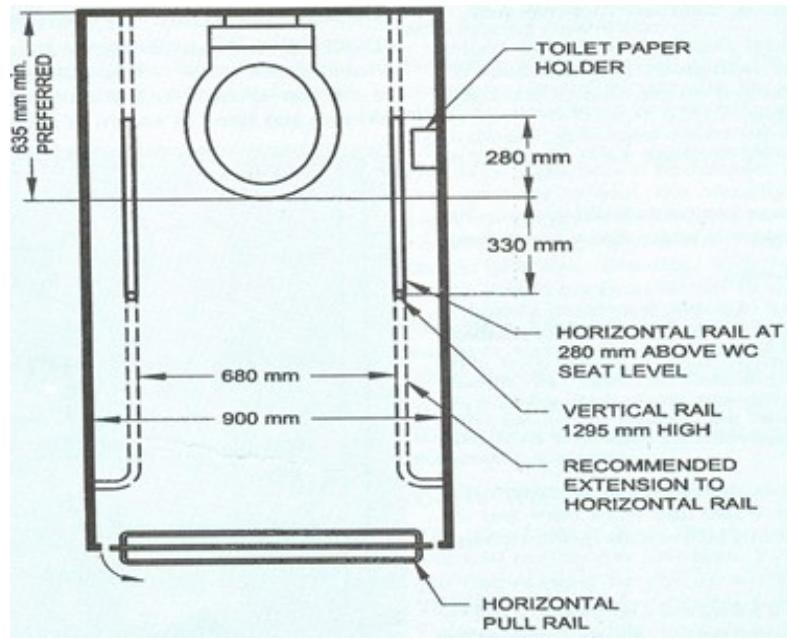
Fig.11 SUGGESTED PLAN WC COMPARTMENT FOR THE AMBULANT
