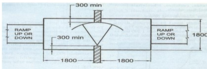
FIG. 3 LEVEL AREAS REQUIRED AT END OF RAMPS LEADING TO DOORWAYS.
