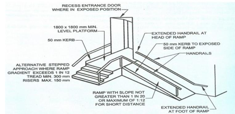
FIG. 2 EXAMPLE OF RAMPED APPROACH
