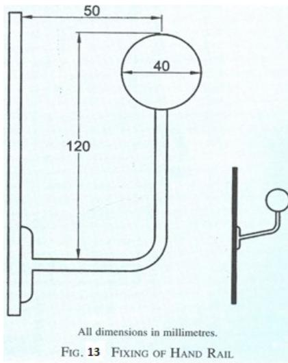
FIG. 13 FIXING OF HAND RAIL
